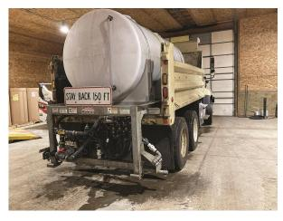
barrier so you don't get ice sticking to the pavement, which makes it a lot easier for blades to get down to the pavement."
